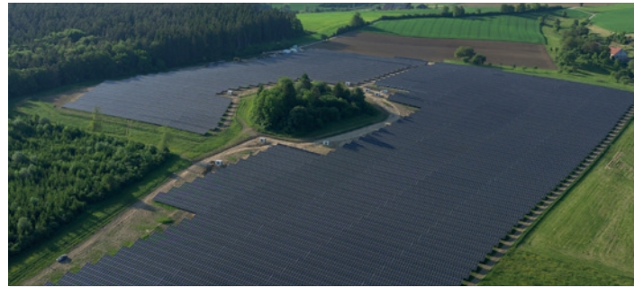
Park: Emmingen, Germany Park size: 17,5 Mwp Mounting system: FMS-V3
